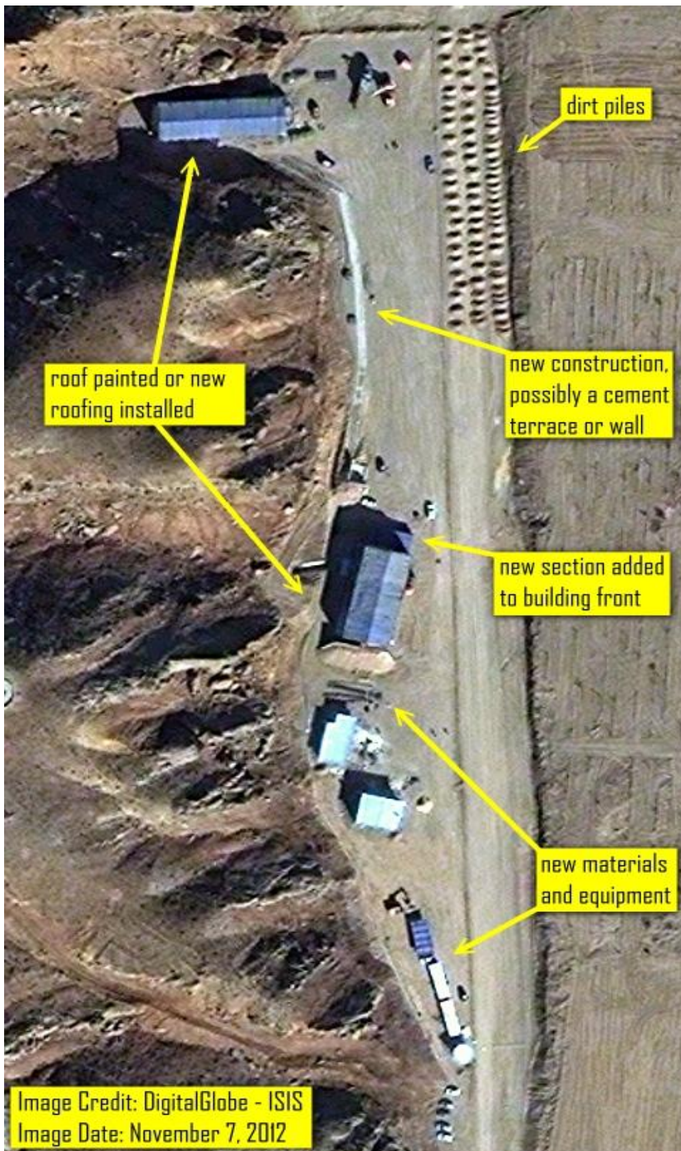
Figure 2: Imagery from November 7, 2012 showing blue roofing covering the two major buildings. An unidentifiable section attached to the front of the suspected chamber building is visible. Rows of earth piles have been collected most likely to be used in paving and construction at the site grounds.
